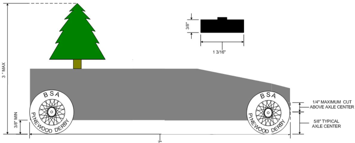
Race cars may be no longer than 7 inches, nor taller than 3 inches, and have an underside clearance of at least 3/8 (0.375) inches. (Rule T-4) & (Rule T-10)
