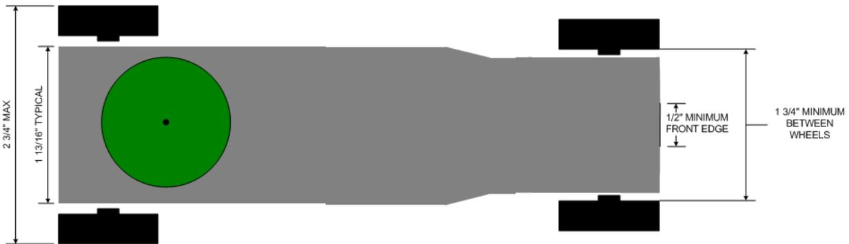
Race cars may be no wider than 2 3/4 (2.75) inches and have inside wheel to wheel clearance of at least 1 3/4 (1.75) inches. The entire car must stage behind the starting pin. The front of the car should have a 1/2" flat surface so it may be accurately placed against the starting pin. (Rule T-4) & (Rule T-10)
